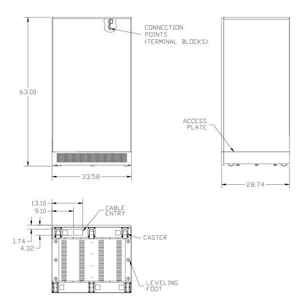
Figure 13 – "F" Battery Cabinet Drawing for 50/80kVA Ratings
